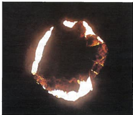
Figure 4. Fayalite maintained at 320 kbar in a Mao-Bell diamond anvil cell. Sample thickness is about 5 \mu\text{m} . Light streaks to the right are reflections from the diamond facets.
