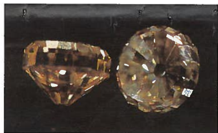
Figure 3. A pair of type I diamonds used for far-IR studies. Largest diameter is 3 mm. Diameter of the tip is 0.6 mm.
