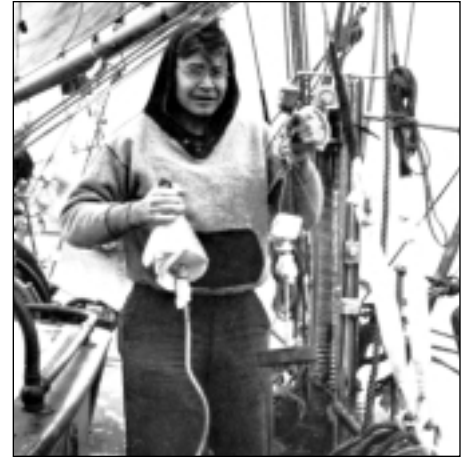
Maurice Ewing was devoted to new and ingenious instruments, such as this timed release mechanism, which was triggered by the dissolution of a block of salt, seen at right. Photo ©Woods Hole Oceanographic Institution. Used with permission.
