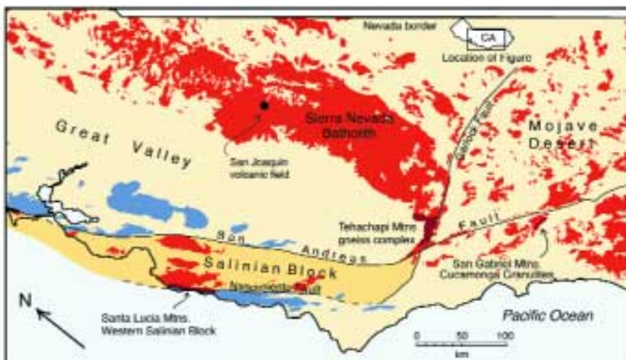
Figure 1. Map of central and southern California (after Jennings, 1977) showing geologic features discussed in text. Mesozoic granitic and related metamorphic rocks are in red. In blue are mainly Jurassic Franciscan formation rocks. Darker red areas show location of Mesozoic arc-related amphibolite-granulite terrains.
