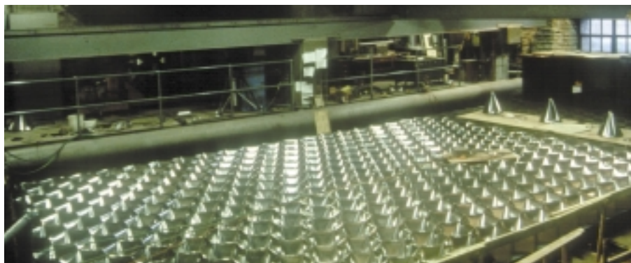
Figure 3. Honeycomb floor of full eXperimental EarthScape (XES) basin, with 432 subsidence cells. A 10-cell version was used for experiment described in this paper.
