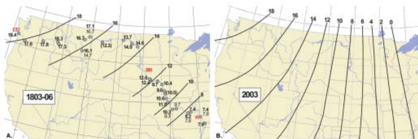
Figure 2. A: Magnetic declination calculated from the solar measurements of Lewis and Clark (bold numbers, Table 2; see footnote 1), based on the latitude and site of observation as determined from their narrative and by comparing modern and historic maps. Numbers represent averages whenever possible, and those given in parentheses indicate irregularities in the reported data; see Table 2 for details. Non-bold numbers represent magnetic declinations utilizing Polaris data (Table 1). Contours are schematic and are based solely on the plotted data. The regular westward increases in magnetic declination strongly support the accuracy of Lewis and Clark’s observations. Locations discussed in the text are K—Kaskaskia, Illinois (Fig. 3); BB—Big Bend, South Dakota (Fig. 4); CD—Cape Disappointment, Washington (Fig. 5). B. Magnetic declination calculated for March 2003 utilizing model IGRF-2000 (U.S. Geological Survey, 2003). The agonic line currently passes through St. Louis County, far west of its location in coastal Virginia ca.1803–1806.
