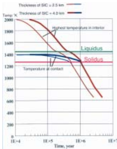
Figure 9. Cooling with time for an impact melt sheets with thicknesses of 2.5 km (thin lines) and 4 km (thick lines). Temperatures at the contact are shown in blue and at the hottest point in the interior in red. Modified after Ivanov and Deutsch (1999). SIC—Sudbury Igneous Complex.
