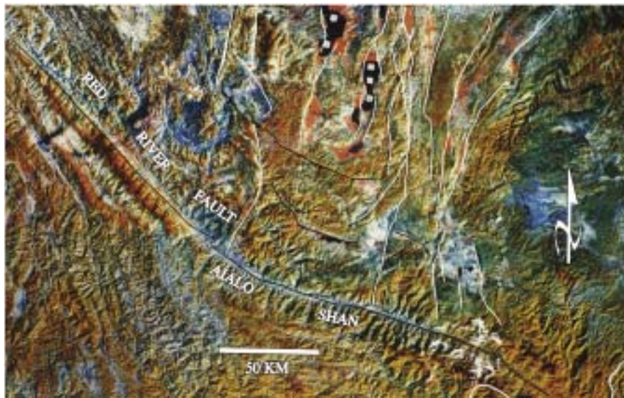
Figure 5. Landsat image of the central part of the Red River area where the left-lateral displacements on faults of the north-south striking Xianshuihe-Xiaojiang fault system, shown in white, die out, but the shear continues across the Red River fault (shown in black), Ailao Shan and structures farther south, bending these features without being marked by prominent surface structures. Two prominent active right-lateral faults north of the Red River fault are also shown in black.
