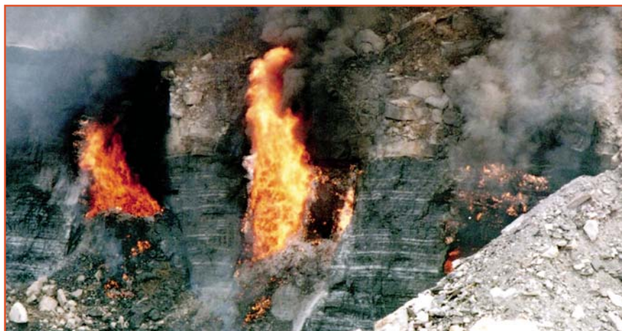
Figure 1. Open-pit mine fire near Dhanbad, Jharia Coalfield, India. Most Jharia fires ignite spontaneously, subsequent to mining. The middle flame is ~7 m (23 ft) high. Source: Daniel B. Sanger, GAI Consultants, Inc., Homestead, Pennsylvania, USA.
