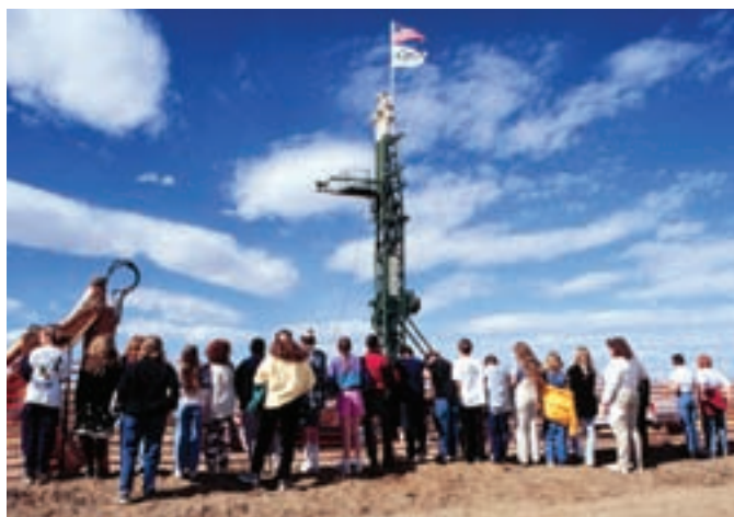
Figure 2. Drilling the Kiowa Core. The rig, operated by Layne Western, recovered over 93% of a 2.5 inch diameter core extending 2256 feet into the basin. Drilling occurred in 1999 and took seven weeks. More than 2000 visitors investigated the round-the-clock drilling operation; as the core was described, curious folks looked over our shoulders for evidence of perforated dinosaurs and other treasures.
