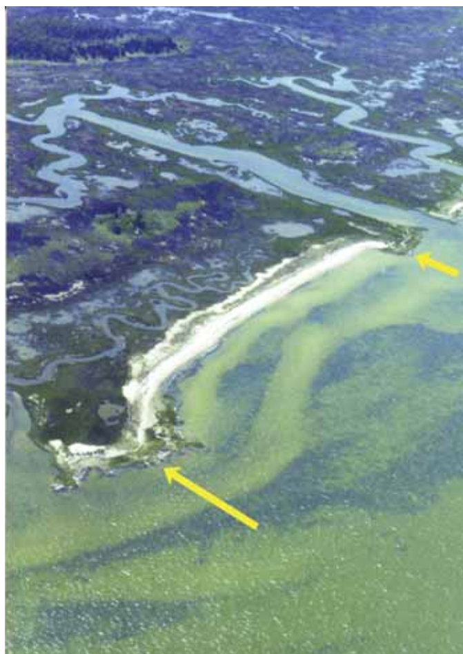
Figure 2. Marsh peat outcrops (marked by arrows) form temporary headlands that control the planform of barrier islands in low-energy settings, such as in this example from Chesapeake Bay.
