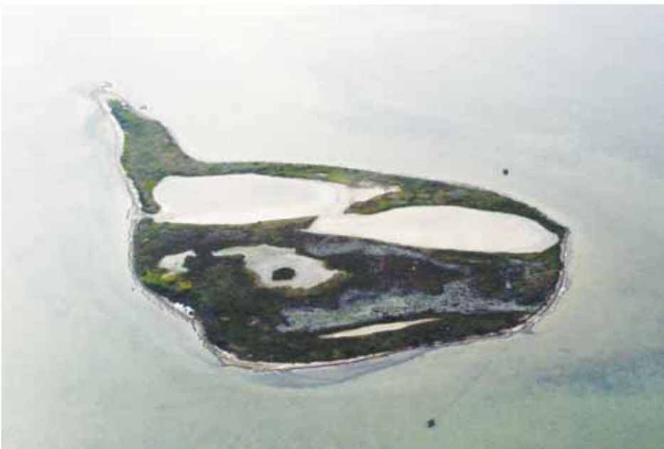
Figure 5. Island in central Laguna Madre, Tamaulipas, México, affected by wave approach from two sides. The resulting fetch-limited sandy barriers, which face opposite directions, have enclosed a central lagoon.
