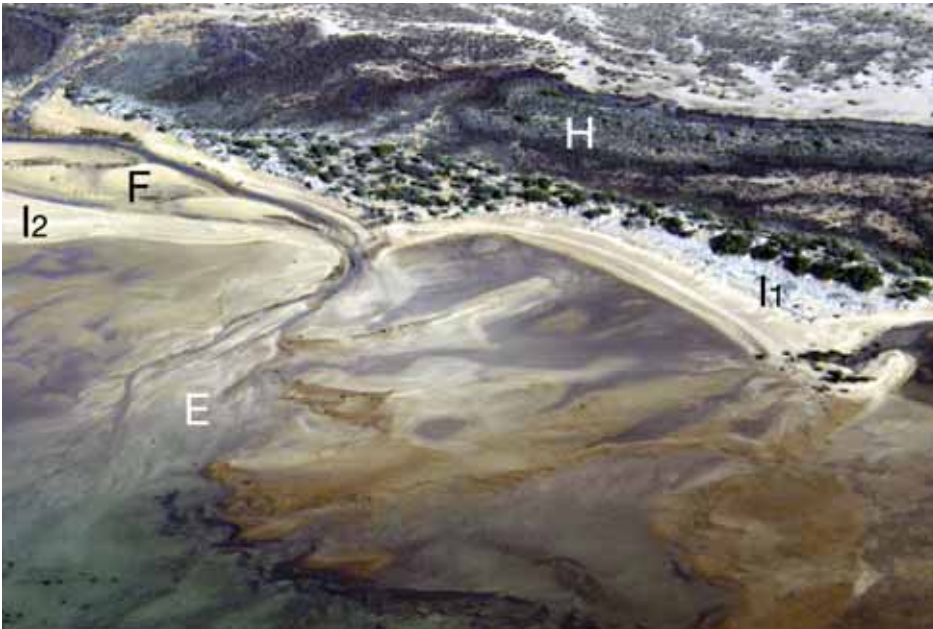
Figure 3. Ebb-tide delta (E) and flood-tide delta (F) developed at a tidal inlet in a fetch-limited barrier island chain (I1, I2) in upper Spencer Gulf, South Australia. The islands are backed by an intermittently flooded supratidal flat (H).
