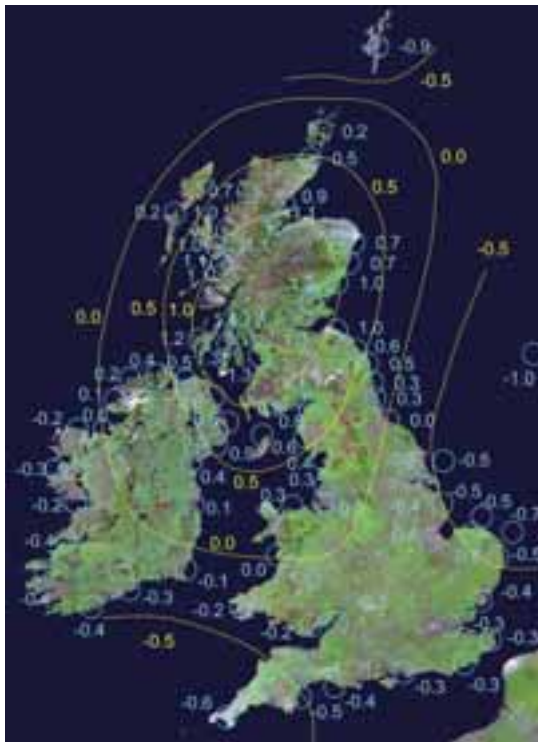
Figure 1. Current rate of relative land- and sea-level change in the British Isles in \text{mm a}^{-1} , showing relative land uplift as positive and relative subsidence as negative. Image is \sim 900 \times 1300 km, courtesy of the NASA Scientific Data Purchase Program.
