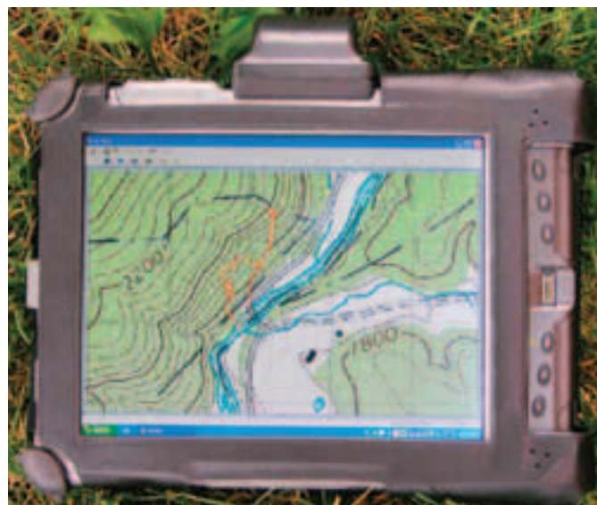
Figure 1. xPlore iX104C tablet PC with ArcPAD field map shown on the screen.
