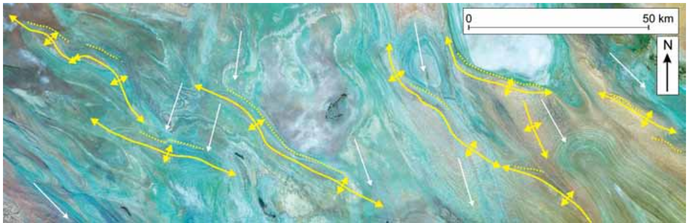
Figure 5. Landsat 7 image of the northwestern Qaidam basin (location shown on Fig. 2A). White arrows—prevailing wind direction during yardang development; yellow lines—axial traces of fault-propagation anticlines; yellow dotted lines—steeper forelimbs of anticlines (perpendicular to propagation direction).
