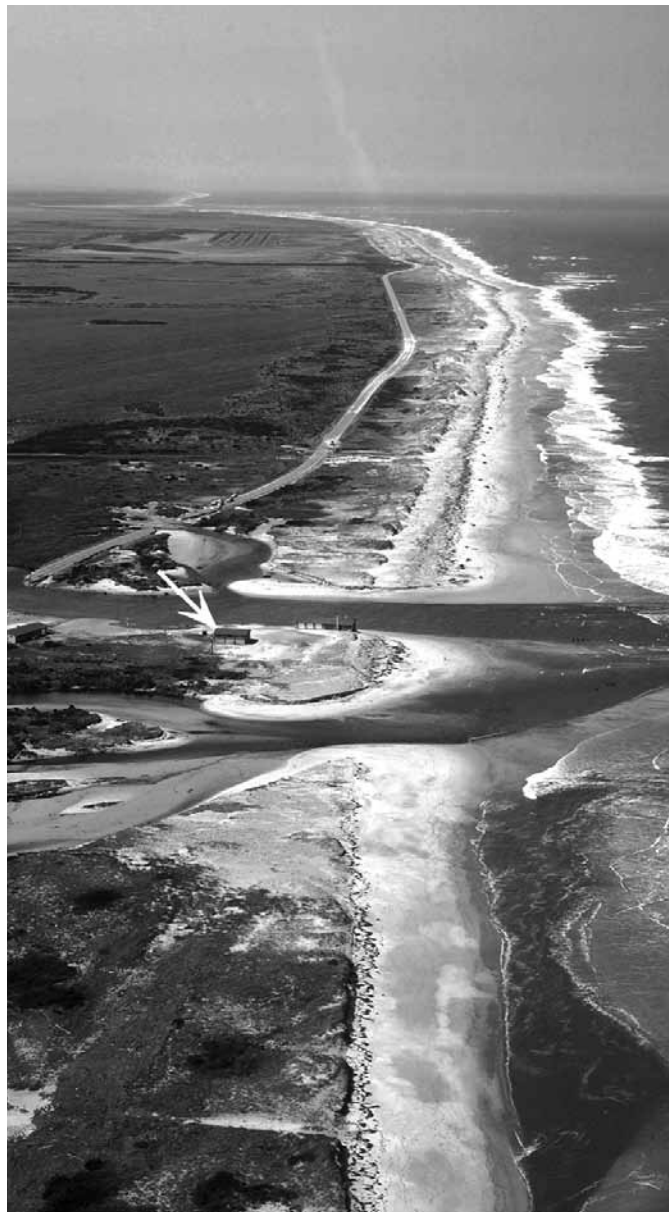
Oblique aerial photograph taken 30 Aug. 2011 of Pea Island National Wildlife Refuge, North Carolina, USA, looking north along the coast. Hurricane Irene made landfall near here on 27 Aug. 2011. At this location, two breaches were carved through the island, severing NC Hwy 12. Arrow points to the Pea Island ranger station. Image courtesy USGS; learn more at http://coastal.er.usgs.gov/hurricanes/irene/photo-comparisons/ .
