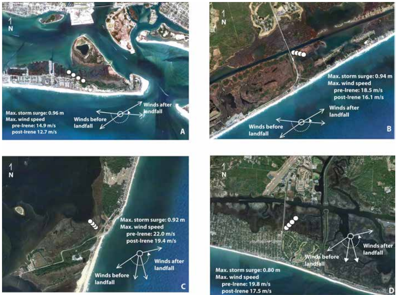
Figure 5. Locations of core samples collected in this study. White dots represent cores taken at each locality; arrows indicate the range of wind directions 24 hours before and 24 hours after landfall of Hurricane Irene. (A) Tar Landing Bay; (B) Alligator Bay; (C) Fort Fisher; (D) Oak Island. Images courtesy Google Earth.
