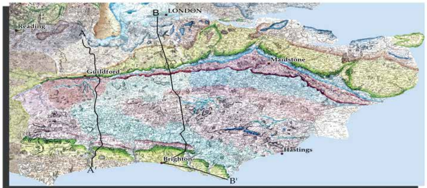
Figure 4. Part of William Smith's 1819 Section of the Strata across Surrey and Sussex shown with part of his 1815 map, which has been draped on an SRTM elevation model. Also shown is a modern composite seismic section (modified from Butler and Jamieson, 2013). Green—Chalk; blue-gray—Greensand and Gault; pink-brown—Purbeck-Portland; blue—older Jurassic; orange-brown—Triassic. The locations of the seismic section (A–A') and Smith's section (B–B') are shown on Smith's county geological maps of Kent, Sussex, and Surrey.
