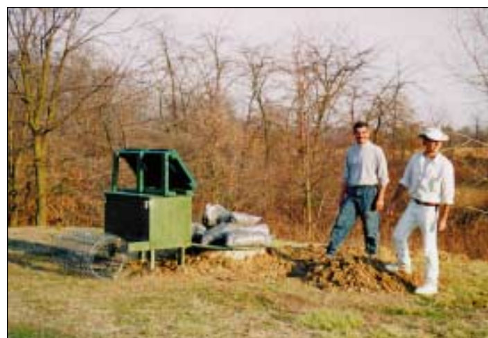
Figure 10. Ghassan Al-Eqabi (left) and Patrick Shore (right) completing installation of one of the MOMA (Missouri-to-Massachusetts) portable-array broad-band seismometers near Lake Newton, Illinois.
