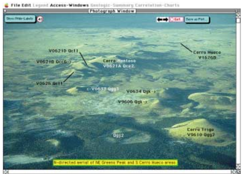
Figure 3. Photograph window of DDM-SVF, showing one of the 74 photos in the program. This oblique aerial photo shows the north-central part of the Springerville field in late afternoon light. A click on the Show/Hide Labels button in the upper left hides all labels. A click on the left or right arrow (upper right) displays the previous or next photo in the program; the Get button lets the user type in the next photo she wishes to view. The photo can be saved as a Pict-format file by clicking on the Save as Pict ... button.
