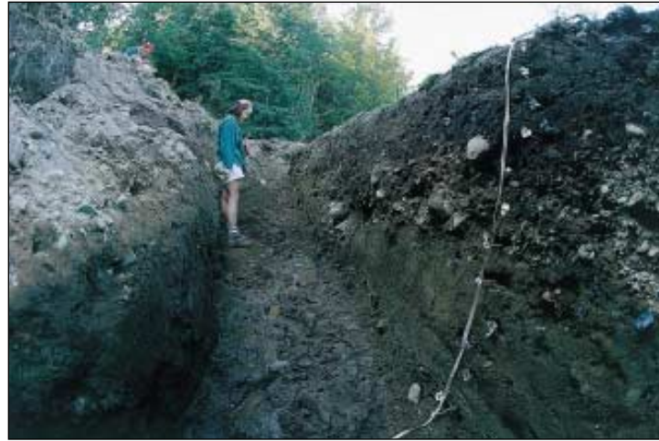
Figure 6. Trench 4 of the Moultroupan fan contains a variety of grain sizes, from silt to cobbles, reflecting different sediment sources, till and glacial lacustrine sediments. The prehistoric soil horizon and overlying postsettlement alluvium are just above the large cobble beyond the tape.
