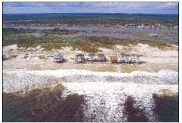
**Figure 5.** Immediately after Hurricane Fran in 1996, an artificial dune was built along the shoreline of North Topsail Beach (the northeastern one-third of Topsail Island) for protection of the only access road. The dune was almost entirely removed by Hurricane Floyd in 1999, and the sand was redistributed as washover deposits on the island.
