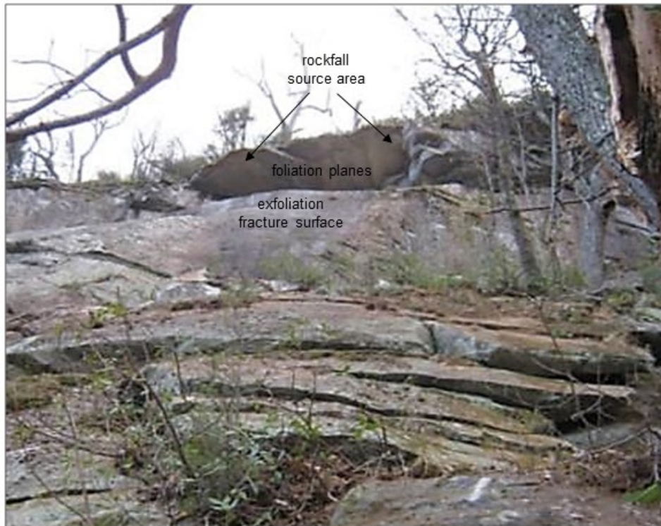
Figure 3-12. Photograph looking upslope toward the rockfall source area. The rock slab detached from an overhang on the cliff face where an exfoliation joint intersects foliation planes in the Henderson Gneiss. 2012/11/19 NCGS photo.
