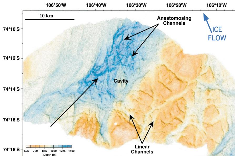
**Figure 6.** Multibeam mosaic showing anastomosing subglacial meltwater channels in inner part of Pine Island Bay.
