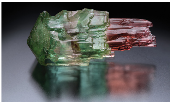
Figure 1. Elbaite crystal, a species of the tourmaline supergroup containing lithium, showing its noncentrosymmetric growth along the long axes (c) which is responsible for its piezoelectric (and pyroelectric) properties, contributing to its utility as a technological material. Color change reflects incorporation of different chemical elements in response to its host environment.
