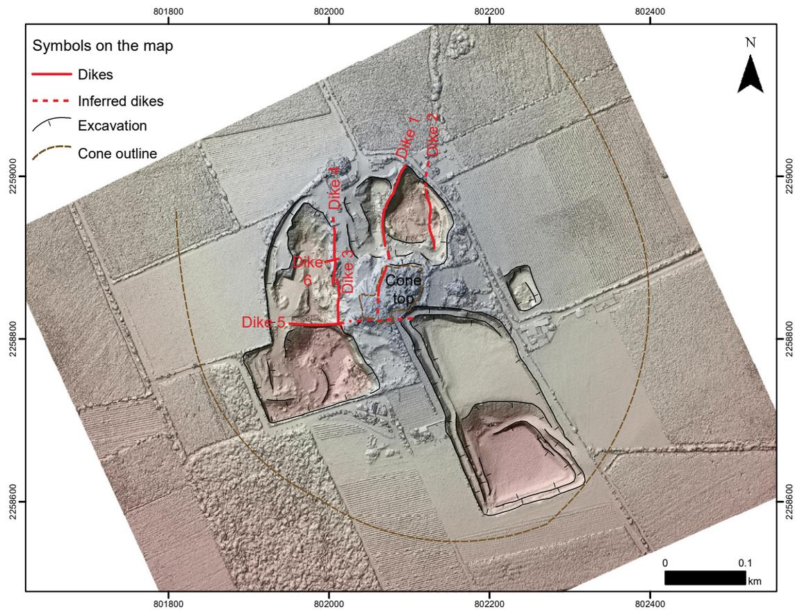
Figure 4. Shaded-relief model of the Cerrito Colorado scoria cone generated with the aerial vehicle. The model allows identifying the quarrying excavation, the exposed dike-feeding system and its cross-cutting relations.
