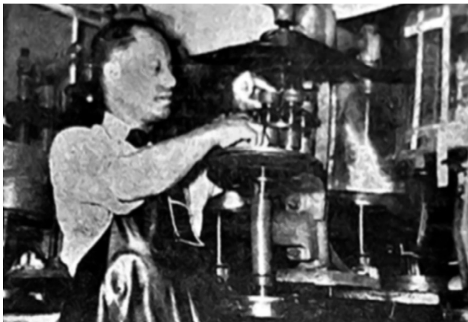
Charles Fletcher loading the Graton-Vanderwilt polishing machine at the Laboratory of Mining Geology at Harvard University. Photo from Boston Globe , 29 November 1954.
