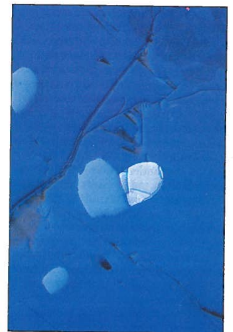
Figure 5. Photomicrograph of coexisting magnetite-pyrrhotite-Cu, Fe monosulfide in a clinopyroxene phenocryst from the July 1992 Galeras andesite (reflected light, Nomarski lens, 0.18 \mu\text{m} field of view).
