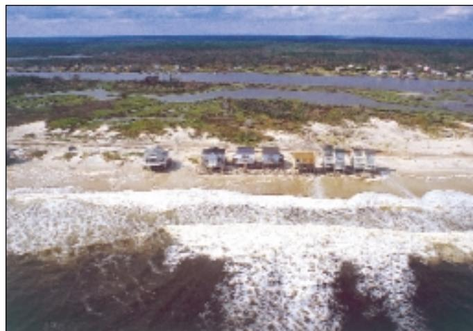
Figure 5. Immediately after Hurricane Fran in 1996, an artificial dune was built along the shoreline of North Topsail Beach (the northeastern one-third of Topsail Island) for protection of the only access road. The dune was almost entirely removed by Hurricane Floyd in 1999, and the sand was redistributed as washover deposits on the island.
