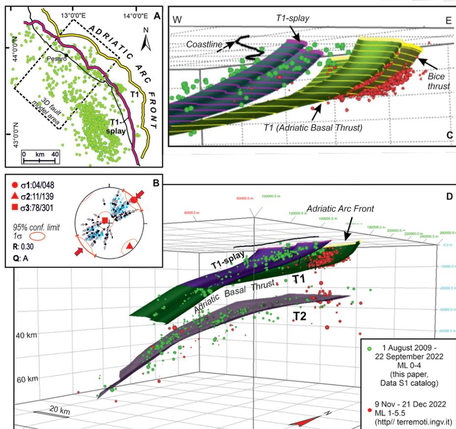
**Figure 3.** Updated 3-D seismotectonic fault model of T1 and T2 megathrusts and T1-splays. (A) OTS EQS Catalog (2009–2022, Fig. S5) with a selection of events (green) associated with T1 and T2. (B) Stress tensor from focal mechanisms associated with T1 and T2 (from de Nardis et al., 2022). (C, D) 3-D view from SE of T1 and T2 with a zoom on Bice thrust and T1-splay. Geometric and kinematic parameters in Fig. S7 (see text footnote 1).
